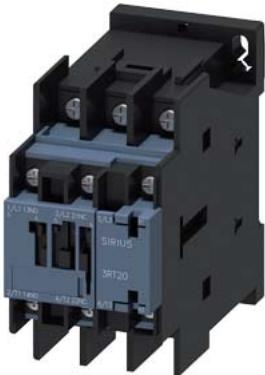
power contactor, AC-3e/AC-3, 25 A, 11 kW / 400 V, 3-pole, 400 V AC, 50 Hz / 400-440 V, 60 Hz, auxiliary contacts: 1 NO + 1 NC, ring cable lug connection, size: S0
