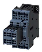
power contactor, AC-3e/AC-3, 25 A, 11 kW / 400 V, 3-pole, 230 V AC, 50/60 Hz, auxiliary contacts: 2 NO + 2 NC, spring-loaded terminal, size: S0, removable auxiliary switch
