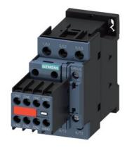
power contactor, AC-3e/AC-3, 25 A, 11 kW / 400 V, 3-pole, 230 V AC, 50/60 Hz, with plugged-in varistor, auxiliary contacts: 2 NO + 2 NC, screw terminal, size: S0, captive auxiliary switch
