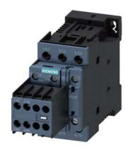
power contactor, AC-3e/AC-3, 25 A, 11 kW / 400 V, 3-pole, 110 V DC, auxiliary contacts: 2 NO + 2 NC, screw terminal, size: S0, removable auxiliary switch
