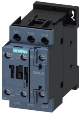
contactor, NEMA version, 5 HP, 460 / 575 V, 3-pole, 110 V AC, 50 Hz / 120 V, 60 Hz, auxiliary contacts: 1 NO + 1 NC, screw terminal, size: S0
