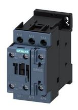
power contactor, AC-3e/AC-3, 25 A, 11 kW / 400 V, 3-pole, 24 V AC, 50 Hz, auxiliary contacts: 1 NO + 1 NC, screw terminal, size: S0, upright mounting position
