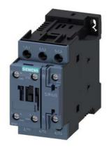
power contactor, AC-3e/AC-3, 17 A, 7.5 kW / 400 V, 3-pole, 200-280 V AC/DC, 50/60 Hz, with integrated varistor, auxiliary contacts: 1 NO + 1 NC, screw terminal, size: S0
