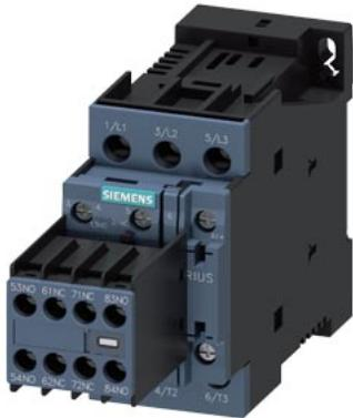
power contactor, AC-3e/AC-3, 17 A, 7.5 kW / 400 V, 3-pole, 24 V DC, with plugged-in diode combination, auxiliary contacts: 3 NO + 3 NC, screw terminal, size: S0, with 3RH2911-1XA22-0MA0
