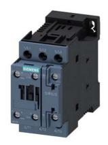
power contactor, AC-3e/AC-3, 17 A, 7.5 kW / 400 V, 3-pole, 72 V DC, auxiliary contacts: 1 NO + 1 NC, screw terminal, size: S0  $\,$
