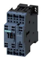
power contactor, AC-3e/AC-3, 9 A, 4 kW / 400 V, 3-pole, 95-130 V AC/DC, 50/60 Hz, with integrated varistor, auxiliary contacts: 1 NO + 1 NC, spring-loaded terminal. size: S0
