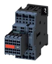
power contactor, AC-3e/AC-3, 9 A, 4 kW / 400 V, 3-pole, 230 V AC, 50/60 Hz, auxiliary contacts: 2 NO + 2 NC, spring-loaded terminal, size: S0, captive auxiliary switch, no surge suppressor retrofittable
