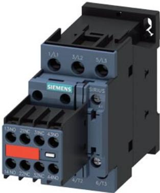
power contactor, AC-3e/AC-3, 9 A, 4 kW / 400 V, 3-pole, 230 V AC, 50/60 Hz, with plugged-in varistor, auxiliary contacts: 2 NO + 2 NC, screw terminal, size: S0, captive auxiliary switch
