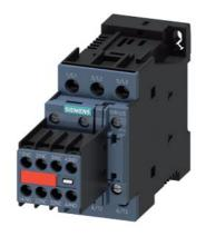
power contactor, AC-3e/AC-3, 9 A, 4 kW / 400 V, 3-pole, 24 V DC, auxiliary contacts: 2 NO + 2 NC, screw terminal, size: S0, captive auxiliary switch, no surge suppressor retrofittable
