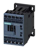
power contactor, AC-3e/AC-3, 16 A, 7.5 kW / 400 V, 3-pole, 24 V AC, 50/60 Hz, auxiliary contacts: 1 NO, spring-loaded terminal, size: S00, upright mounting position
