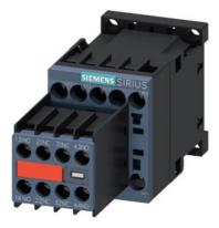
power contactor, AC-3e/AC-3, 16 A, 7.5 kW / 400 V, 3-pole, 24 V DC, auxiliary contacts: 2 NO + 2 NC, screw terminal, size: S00, captive auxiliary switch
