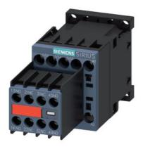
power contactor, AC-3e/AC-3, 16 A, 7.5 kW / 400 V, 3-pole, 110 V AC, 50 Hz / 120 V, 60 Hz, auxiliary contacts: 2 NO + 2 NC, screw terminal, size: S00, captive auxiliary switch
