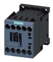
contactor, NEMA version, 5 HP, 460 / 575 V, 3-pole, 24 V AC, 50/60 Hz, auxiliary contacts: 1 NO, screw terminal, size: S00
