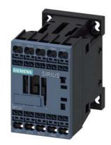
power contactor, AC-3e/AC-3, 12 A, 5.5 kW / 400 V, 3-pole, 24 V DC, 0.85-1.85  $^{\star}$  Us, with integrated suppressor diode, auxiliary contacts: 1 NO, spring-loaded terminal, size: S00
