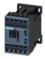
power contactor, AC-3e/AC-3, 12 A, 5.5 kW / 400 V, 3-pole, 24 V DC, 0.7-1.25\* Us, with integrated varistor, auxiliary contacts: 1 NC, spring-loaded terminal, size: S00
