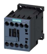
power contactor, AC-3e/AC-3, 12 A, 5.5 kW / 400 V, 3-pole, 24 V DC, 0.85-1.85  $^{\star}$  Us, with integrated suppressor diode, auxiliary contacts: 1 NO, screw terminal, size: S00
