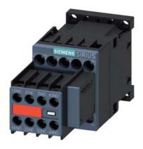
power contactor, AC-3e/AC-3, 12 A, 5.5 kW / 400 V, 3-pole, 230 V AC, 50/60 Hz, with varistor plugged on, auxiliary contacts: 2 NO + 2 NC, screw terminal, size: S00, captive auxiliary switch
