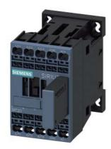
power contactor, AC-3e/AC-3, 9 A, 4 kW / 400 V, 3-pole, 24 V DC, 0.7-1.25\* Us, with varistor plugged on, auxiliary contacts: 1 NC, spring-loaded terminal, size: S00, not expandable with auxiliary switch
