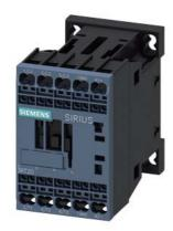
power contactor, AC-3e/AC-3, 9 A, 4 kW / 400 V, 3-pole, 24 V DC, 0.7-1.25\* Us, auxiliary contacts: 1 NO, spring-loaded terminal, size: S00, suitable for PLC outputs, not expandable with auxiliary switch
