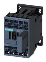
power contactor, AC-3e/AC-3, 9 A, 4 kW / 400 V, 3-pole, 24 V DC, with varistor plugged on, auxiliary contacts: 1 NO, spring-loaded terminal, size: S00, upright mounting position
