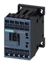
power contactor, AC-3e/AC-3, 9 A, 4 kW / 400 V, 3-pole, 42 V AC, 50/60 Hz, auxiliary contacts: 1 NO, spring-loaded terminal, size: S00
