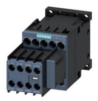
power contactor, AC-3e/AC-3, 9 A, 4 kW / 400 V, 3-pole, 110 V AC, 50/60 Hz, with varistor plugged on, auxiliary contacts: 3 NO + 2 NC, screw terminal, size: S00, removable auxiliary switch
