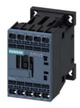
power contactor, AC-3e/AC-3, 7 A, 3 kW / 400 V, 3-pole, 24 V DC, 0.7-1.25\* Us, with integrated diode, auxiliary contacts: 1 NO, spring-loaded terminal, size: S00, suitable for PLC outputs, not expandable with auxiliary switch , reusable packaging, pack = 120 units
