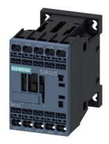
power contactor, AC-3e/AC-3, 7 A, 3 kW / 400 V, 3-pole, 125 V DC, auxiliary contacts: 1 NC, spring-loaded terminal, size: S00  $\,$
