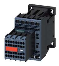
power contactor, AC-3e/AC-3, 7 A, 3 kW / 400 V, 3-pole, 110 V DC, auxiliary contacts: 1 NO + 3 NC, spring-loaded terminal, size: S00, captive auxiliary switch, center auxiliary NC contact current path unequipped
