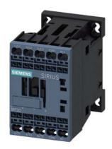
power contactor, AC-3e/AC-3, 7 A, 3 kW / 400 V, 3-pole, 24 V DC, auxiliary contacts: 1 NC, spring-loaded terminal, size: S00, reusable packaging, pack = 120 units
