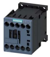
power contactor, AC-3e/AC-3, 7 A, 3 kW / 400 V, 3-pole, 24 V AC, 50/60 Hz, auxiliary contacts: 1 NO, screw terminal, size: S00, suspended mounting position
