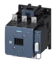
power contactor, AC-3e/AC-3 400 A, 200 kW / 400 V AC (50-60 Hz) / DC Uc: 96-127 V PLC input 24 V DC 3-pole, auxiliary contacts 1 NO + 1 NC drive: electronic main circuit: busbar control and auxiliary circuit: screw terminal with remaining lifetime indicator
