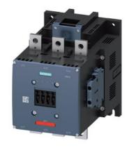
power contactor, AC-3e/AC-3 400 A, 200 kW / 400 V AC (50-60 Hz) / DC Uc: 220-240 V 3-pole, auxiliary contacts 2 NO + 2 NC permanently mounted drive: conventional main circuit: busbar control and auxiliary circuit: screw terminal
