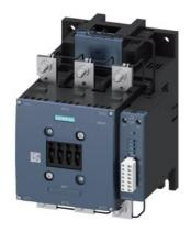
power contactor, AC-3e/AC-3 300 A, 160 kW / 400 V, AC (50-60 Hz) / DC Uc: 200-277 V PLC input 24 V DC 3-pole, auxiliary contacts 1 NO + 1 NC drive: electronic main circuit: busbar control and auxiliary circuit: screw terminal with remaining lifetime indicator
