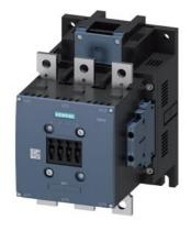
Power contactor, AC-3 300 A, 160 kW / 400 V AC (50-60 Hz) / DC operation 23-26 V AC/DC Auxiliary contacts 2 NO + 2 NC 3-pole, Size S10 Busbar connections Drive: conventional screw terminal NEMA version
