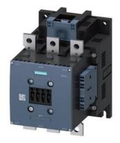
power contactor, AC-3e/AC-3 265 A, 132 kW / 400 V AC (50-60 Hz) / DC Uc: 21-27, 3 V PLC input 24 V DC 3-pole, auxiliary contacts 2 NO + 2 NC drive: electronic main circuit: busbar control and auxiliary circuit: spring-loaded terminal
