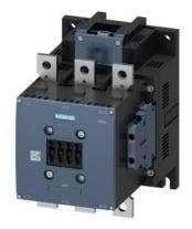
power contactor, AC-3e/AC-3 225 A, 110 kW / 400 V AC (50-60 Hz) / DC Uc: 21-27.3 V PLC input 24 V DC 3-pole, auxiliary contacts 2 NO + 2 NC drive: electronic main circuit: busbar control and auxiliary circuit: screw terminal
