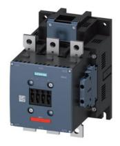
power contactor, AC-3e/AC-3 225 A, 110 kW / 400 V AC (50-60 Hz) / DC Uc: 23-26 V 3-pole, auxiliary contacts 2 NO + 2 NC permanently mounted drive: conventional main circuit: busbar control and auxiliary circuit: screw terminal
