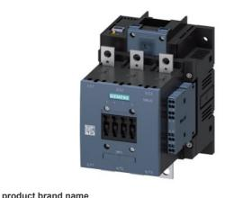
power contactor, AC-3e/AC-3 185 A, 90 kW / 400 V AC (50-60 Hz) / DC Uc: 200-277 V PLC input 24 V DC 3-pole, auxiliary contacts 2 NO + 2 NC solid-state compatible drive: electronic main circuit: busbar control and auxiliary circuit: screw terminal
