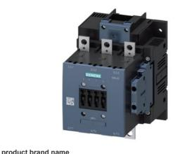
contactor, 100HP, 460 / 575 V AC (50...60 Hz) / DC operation 23 ... 26 V AC/DC auxiliary contacts 2 NO + 2 NC 3-pole, frame size S6 busbar connections drive: conventional NEMA size 4
