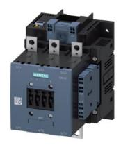
power contactor, AC-3e/AC-3 185 A, 90 kW / 400 V AC (50-60 Hz) / DC Uc: 96-127 V PLC input 24 V DC 3-pole, auxiliary contacts 2 NO + 2 NC drive: electronic main circuit: busbar control and auxiliary circuit: spring-loaded terminal
