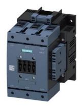
power contactor, AC-3e/AC-3 150 A, 75 kW / 400 V AC (50-60 Hz) / DC Uc: 23-26 V 3-pole, auxiliary contacts 2 NO + 2 NC drive: conventional main circuit: box terminal control and auxiliary circuit: screw terminal box terminal up to 70  $\,\mathrm{mm^2}$
