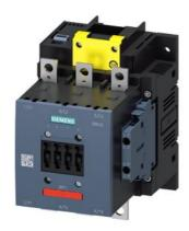
power contactor, AC-3e/AC-3 150 A, 75 kW / 400 V AC (50-60 Hz) / DC Uc: 200-277 V x (0.8-1.1) F-PLC input 24 V DC 3-pole, auxiliary contacts 2 NO + 2 NC permanently mounted drive: electronic main circuit: busbar control and auxiliary circuit: screw terminal
