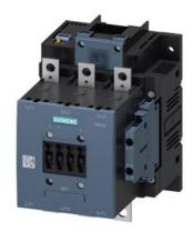
power contactor, AC-3e/AC-3 150 A, 75 kW / 400 V AC (50-60 Hz) / DC Uc: 96-127 V PLC input 24 V DC 3-pole, auxiliary contacts 2 NO + 2 NC drive: electronic main circuit: busbar control and auxiliary circuit: screw terminal
