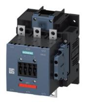
power contactor, AC-3e/AC-3 150 A, 75 kW / 400 V AC (50-60 Hz) / DC Uc: 220-240 V 3-pole, auxiliary contacts 2 NO + 2 NC permanently mounted drive: conventional main circuit: busbar control and auxiliary circuit: screw terminal
