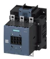
power contactor, AC-3e/AC-3 150 A, 75 kW / 400 V AC (50-60 Hz) / DC Uc: 220-240 V 3-pole, without auxiliary contacts drive: conventional main circuit: busbar control and auxiliary circuit: screw terminal
