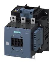
power contactor, AC-3e/AC-3 115 A, 55 kW / 400 V, AC (50-60 Hz) / DC Uc: 21-27.3 V PLC input 24 V DC 3-pole, auxiliary contacts 2 NO + 2 NC drive: electronic main circuit: busbar control and auxiliary circuit: spring-loaded terminal
