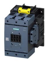
power contactor, AC-3e/AC-3 115 A, 55 kW / 400 V, AC (50-60 Hz) / DC Uc: 96-127 V x (0.8-1.1) F-PLC input 24 V DC 3-pole, auxiliary contacts 2 NO + 2 NC drive: electronic main circuit: box terminal control and auxiliary circuit: screw terminal
