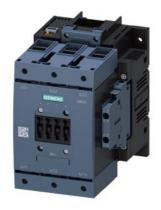
power contactor, AC-3e/AC-3 115 A, 55 kW / 400 V, AC (50-60 Hz) / DC Uc: 96-127 V PLC input 24 V DC 3-pole, auxiliary contacts 2 NO + 2 NC drive: electronic main circuit: box terminal control and auxiliary circuit: screw terminal
