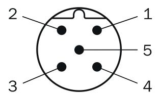
Connector M12, 5-pin, A-coded
